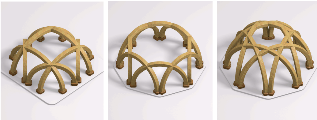
Figure 13. Rendering of the 3 types of ribbed domes: lattice + diamond, and stars [8/2] and [8/3].
