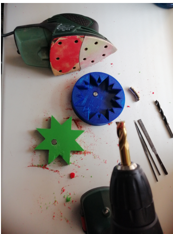
Figure 36. Post-processing works on the pieces: sanding and attaching magnets.
